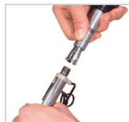
Rotate anticlockwise and release the tool ring
